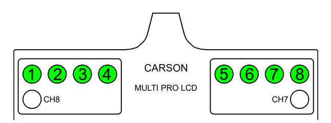
For the switches 1 - 8 two functions can be assigned in the Sound-Teacher or in the Drive-Teacher. One function for "switch up" and one function for "switch down". In total 16 additional functions can be switches with the MSC-8-C-LCD.
