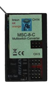
Channel CH5, CH6 and CH9 - CH14 are used by the MSC. These channels can not be used for additional functions, such as servos, speed controler or switching modules!
