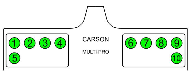
For the switches 1 - 10 two functions can be assigned in the Sound-Teacher or in the Drive-Teacher. One function for "switch up" and one function for "switch down". In total 20 additional functions can be switches with the MSC-10-C.
