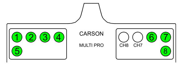
For the switches 1 - 8 two functions can be assigned in the Sound-Teacher or in the Drive-Teacher. One function for "switch up" and one function for "switch down". In total 16 additional functions can be switches with the MSC-8-C.
